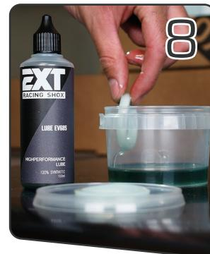
Fill a small container with the EXT EV68S oil that's used to lubricate the lowers.
