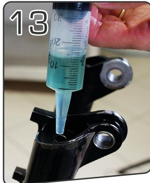
Using a syringe, insert the correct volume of oil into the lowers:
