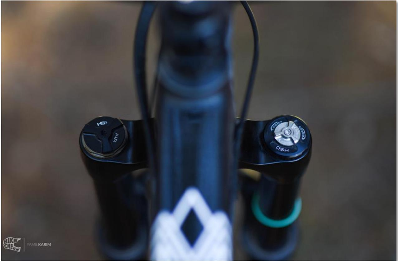
The cartridge features high speed, low speed and rebound compression settings. You'll have many adjustments that will help you to adapt the ERA to your taste, type of handling and terrain.
