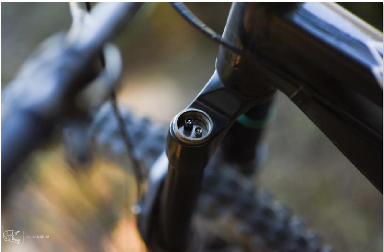
It has two positive air chambers and one high volume negative chamber. These two positive chambers allow us to infinitely adjust the medium support and the progressivity of its travel, while the high-volume negative chamber gives us a feeling very similar to that of a spring.
